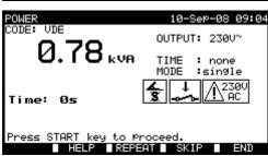
Functional test – apparent power measurement
