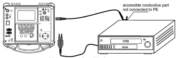
Measurement of touch leakage current
