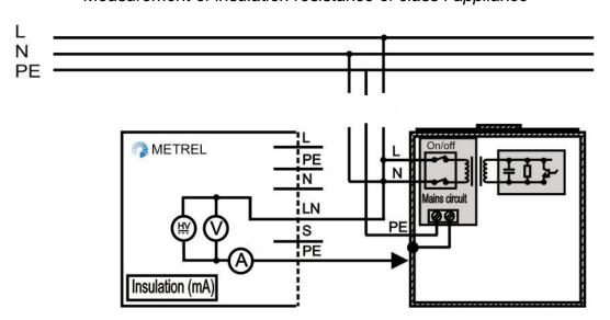
Measurement of insulation resistance of fixed installed appliances of Class I
