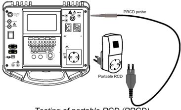
Testing of portable RCD (PRCD)
