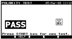
Example of polarity test result
