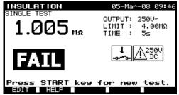
Examples of insulation resistance measurement results
