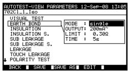
Modification parameters of selected test function
