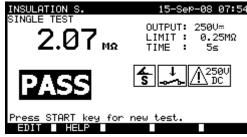
Example of insulation S. resistance measurement results
