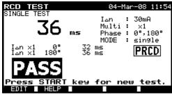
Example of RCD test result
