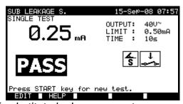
Example of substitute leakage current measurement results
