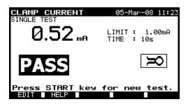
Example of clamp current measurement result
