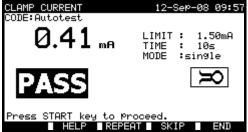
TRMS current measurement using current clamps
