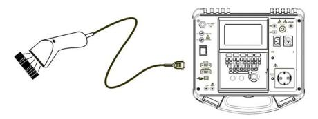
Connecting barcode reader to the OmegaGT Plus / BetaGT Plus instrument
