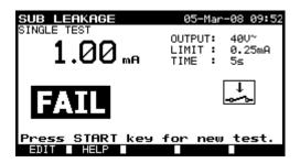
Examples of substitute leakage current measurement results
