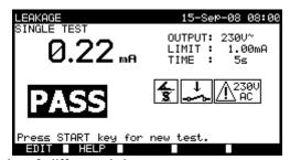
Example of differential current measurement result
