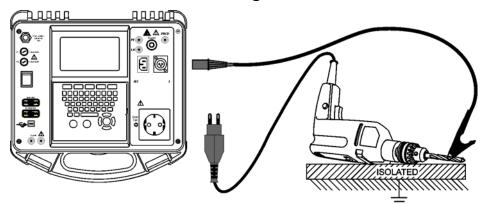
Measurement of substitute leakage current of class II appliance
