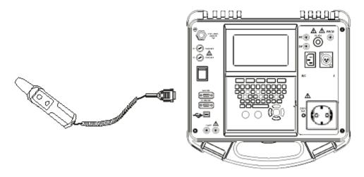
Connecting RFID tag reader/writer to the OmegaGT Plus / BetaGT Plus instrument
