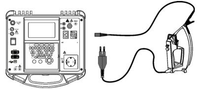
Measurement of earth bond resistance of class I appliance
