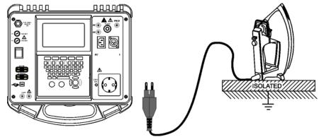
Measurement of substitute leakage current of class I appliance
