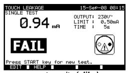
Examples of touch leakage current measurement results (slika)
