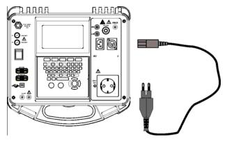
Polarity test of IEC cord
