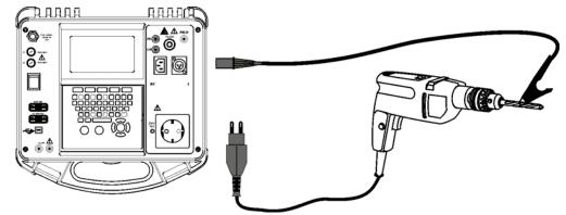
Measurement of insulation resistance of class II appliance
