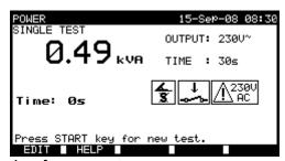
Example of apparent power measurement result
